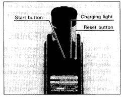
goes out within 10 seconds even after pressing the reset button and start button a couple of times, the battery cartridge is dead. (CAUTION: Wait for more than 5 seconds after the charging light goes out to press the reset button again.) Replace it with a new one. When the charging light goes out after about one hour, you may remove the fully charged battery cartridge.
